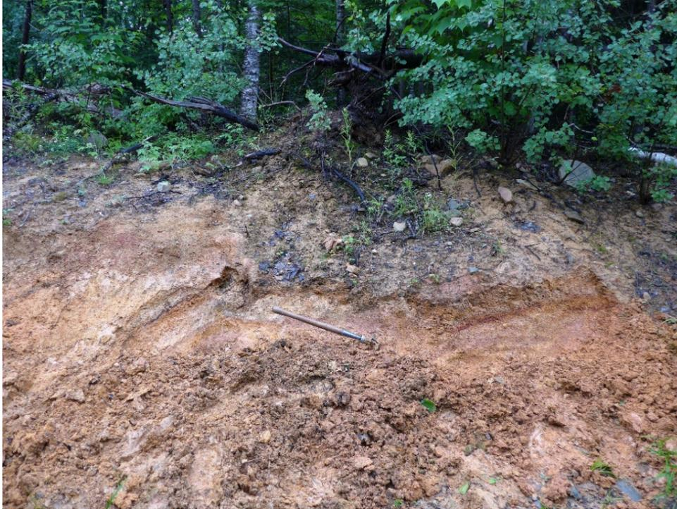
**Figure 15.** Clay exposure at Stop 7-A. The stones on upper part of section probably were introduced by road work.
