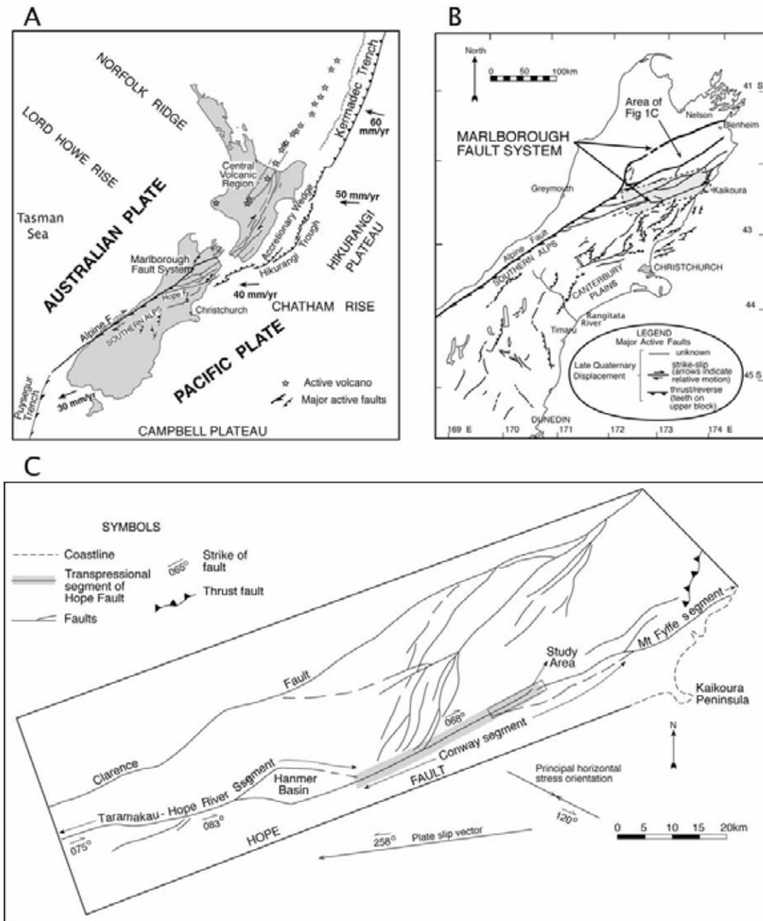
**Figure 1:** Location of the study area and general tectonic setting of the Hope Fault; A, Regional tectonic setting of New Zealand. B, Marlborough Fault System in the South Island. C, Hope Fault showing the strike of various segments of the fault, the Pacific plate motion vector, and principal horizontal stress orientation from Pettinga & Wise (1994) and Nicol & Van Dissen (2002).
