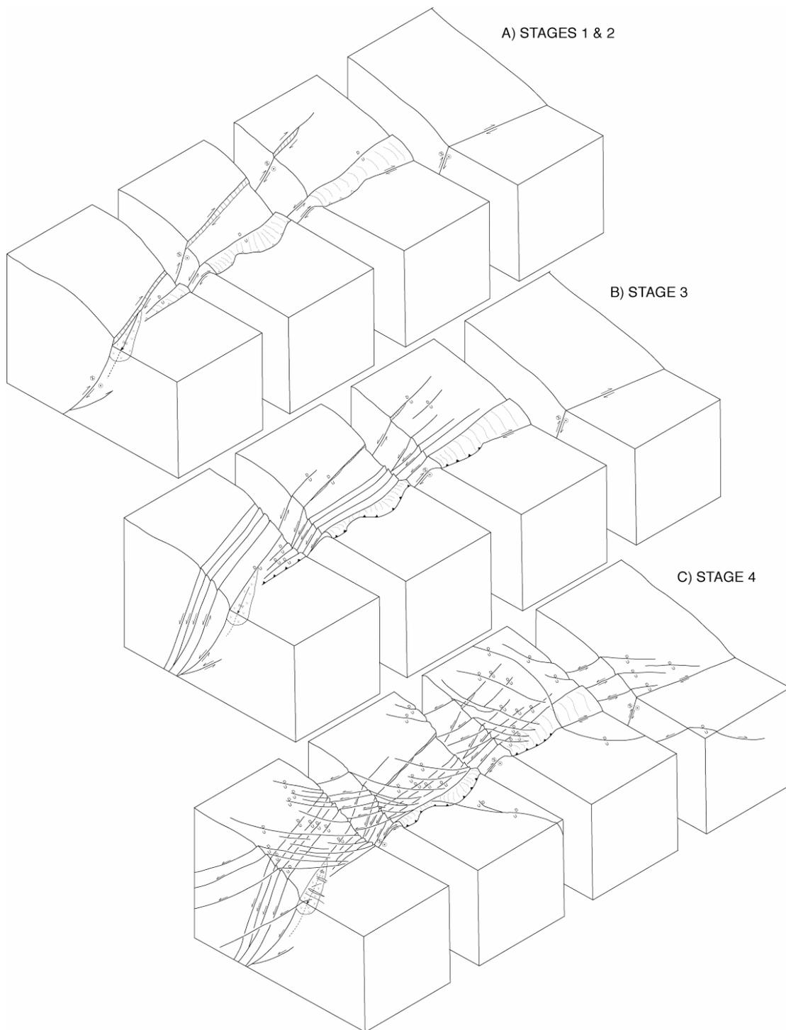
**Figure 5:** Three-dimensional schematic model for the development and modification of the Hope Fault in the Charwell River area. A, Stage 1 and 2 formation of the initial fault wedge. B, Stage 3, collapse of the initial wedge along normal faults parallel to the central segment of the Hope Fault. C, Initiation of the secondary fault wedge and late normal faults due to collapse of the entire hanging wall (from Eusden et al. 2005).
