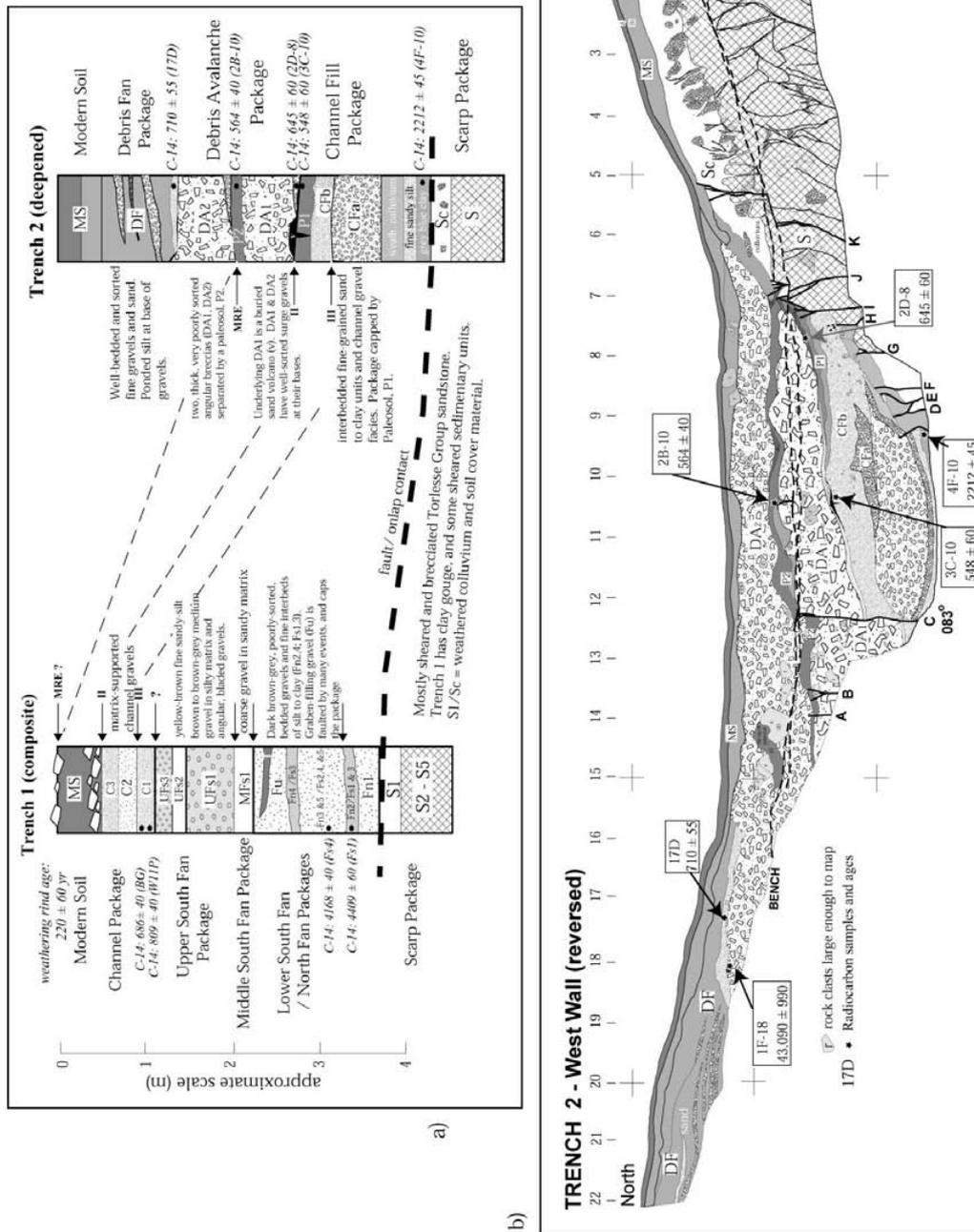
**Figure 8:** a) Summary of stratigraphy and dates from Trenches 1 and 2 at Greenburn Stream. Arrows and Roman numbers refer to earthquake event horizon positions. b) log of West wall of Trench 2 (modified after Langridge et al 2003). After deepening within the central fault zone and basin, further event horizon, age control and a liquefaction sand source were discovered.
