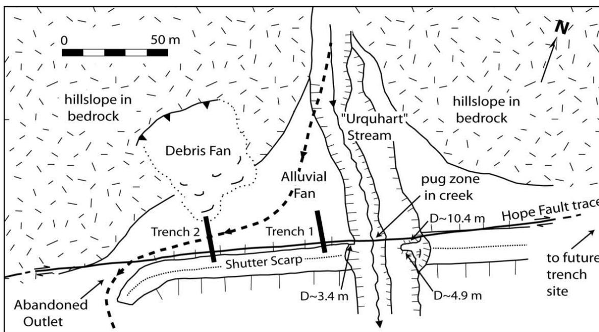
**Figure 7:** Geomorphic map of the Greenburn Stream trench site (modified after Pope 1994). Modern incised Urquhart Stream crosses the fault but was formally dextrally deflected by 100-130 m and drained through the abandoned outlet. Small dextral displacements and the pug zone of the fault can be observed in the floor of the modern stream.
