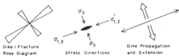
Figure 4.7 Image from McHone's (1988) paper, illustrating what extensional features would form from a given stress orientation, and in which direction these features would propagate (McHone, 1988).
