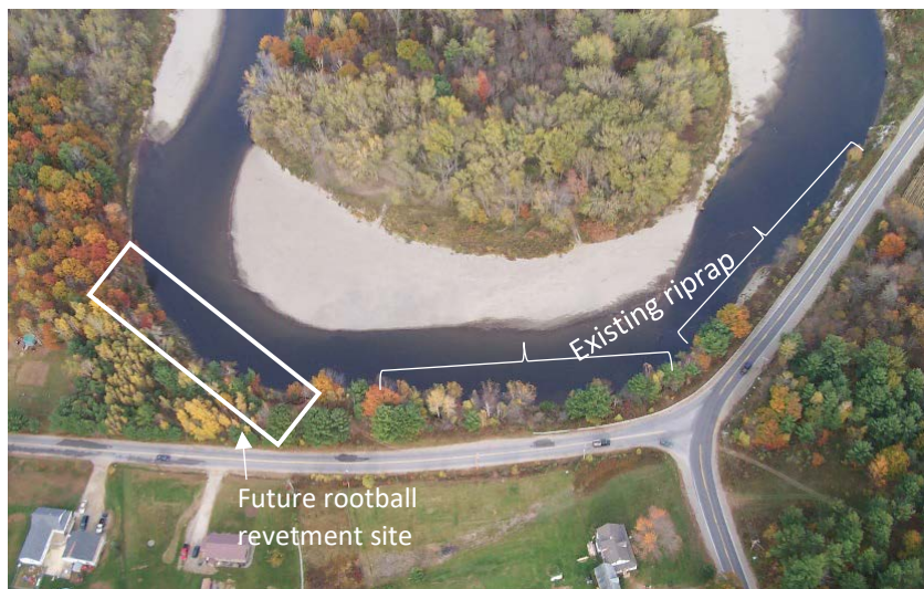
Figure 12. View of the Meader Bar in fall, 2011. Older riprap along Rt. 156 is indicated, and the extensive upstream point bar is in the center of the photo. River flow is from left to right. The future site of the rootball revetment constructed to protect Whittier Road is outlined.
