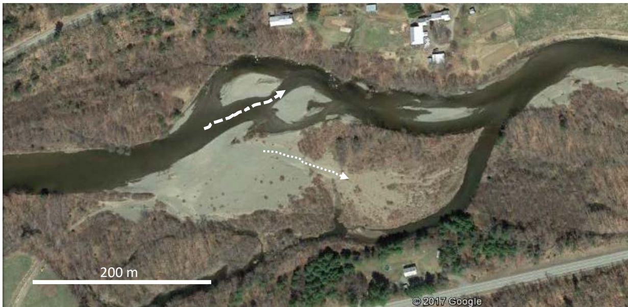
Figure 8. The most recent Google Earth image of Voter Bar, acquired in 2016 (Google Earth, 2017). The main channel now follows only the dashed arrow. Prior to sand and gravel removal, the main channel was adjacent to the cutbank on the north side. A prominent chute, used during highwater flows, is shown by the dotted arrow. This path would have been the presumed new channel had the river migrated naturally.
