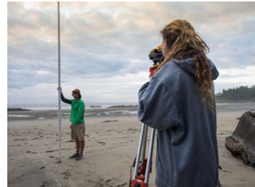
Figure. 2.2 Autolevel survey method.
