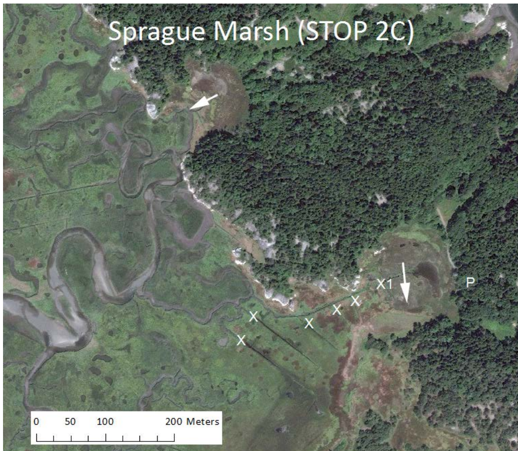
Figure 13. Points of interest at STOP 2C, where P = parking area, X1 = largest ditchplug, other X = other ditchplugs. White arrows represent direction of groundwater flow in two similar alcoves along the margins of the marsh (from Barry, 2012). (Satellite image taken 8/15/13.)
