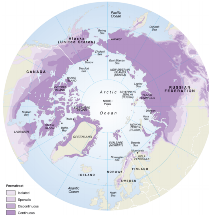
Figure 1.1: Northern Hemisphere spatial distribution of permafrost where, tan represents permafrost free areas and shades of purple represent regions of isolated, sporadic, discontinuous, or continuous permafrost cover. Figure from Schuur et al. 2008.
