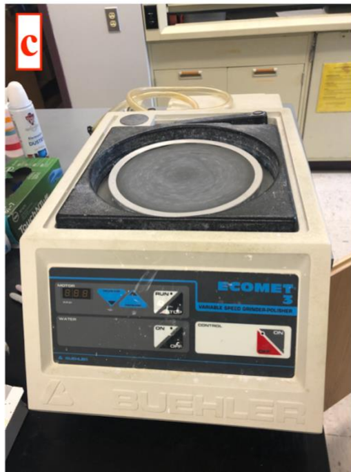
Figure 2.2 a) Braun Chipmunk rock crusher (right) and Bico, Inc. rock pulverizer (left). b) Spex Industries, Inc. mixer/mill. c) Ecomet 3 variable speed grinder-polisher with 600 grit sandpaper.
