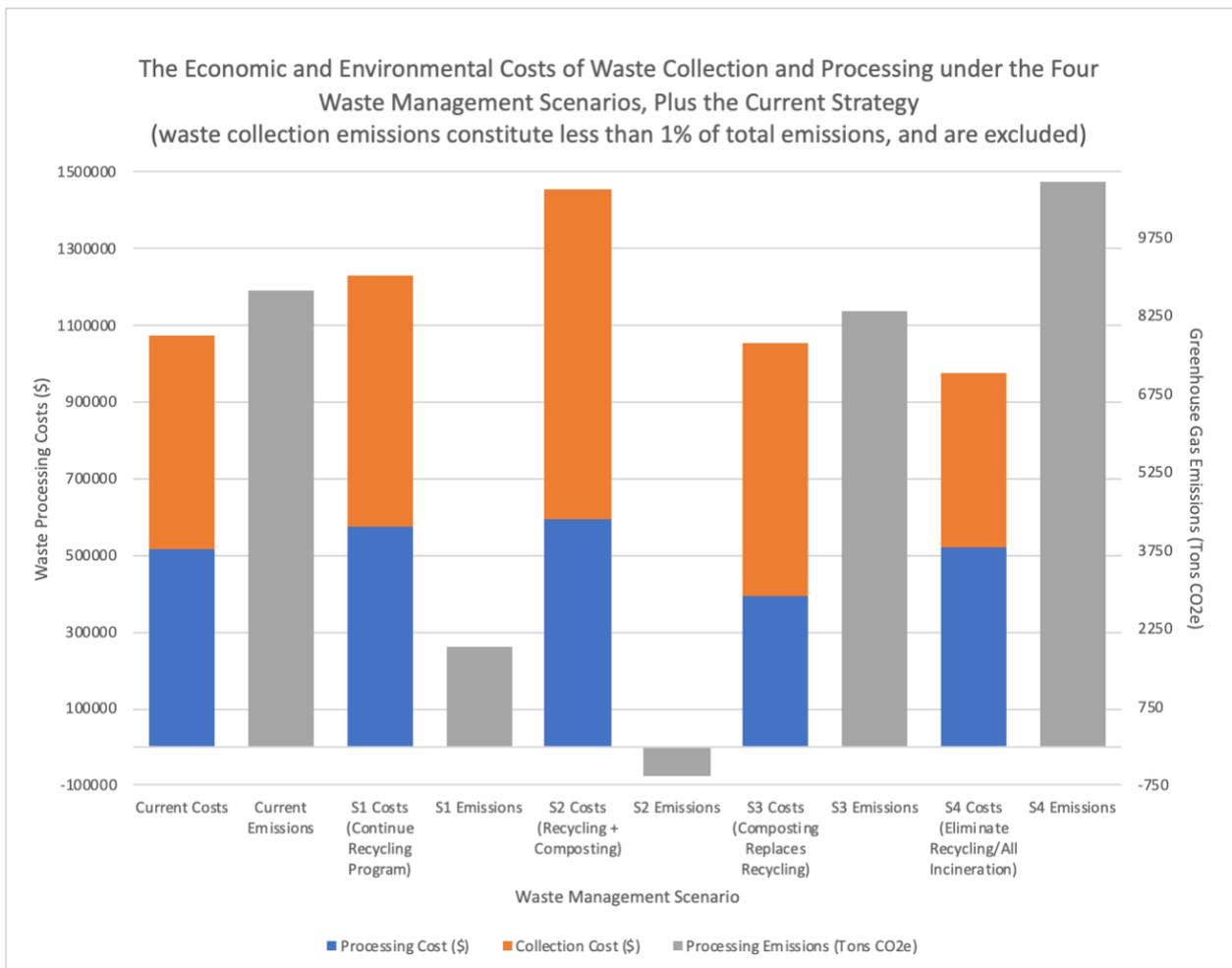
Figure 6: The economic and environmental costs of waste collection and processing under the four scenarios.
