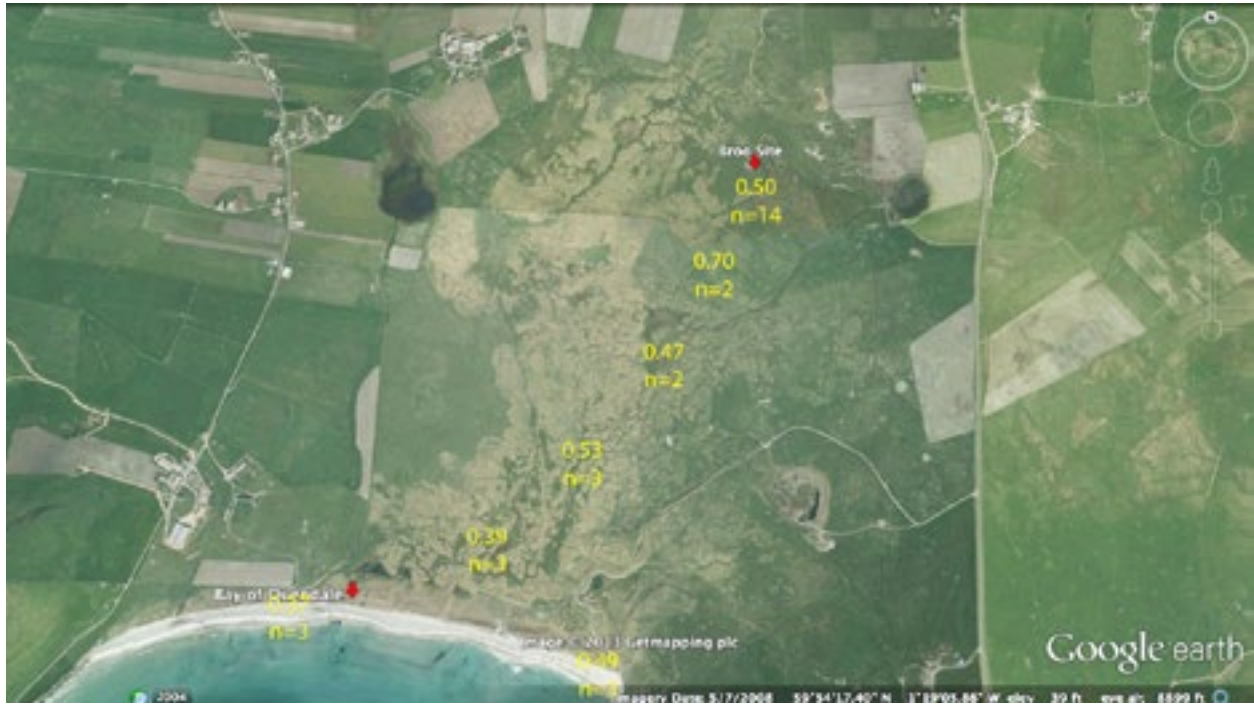
Figure 29: Average inclusive graphic standard deviation values (in units phi) for the Bay of Quendale, the Quendale Transect, and the Broo archaeological site. Note: lower values indicate better sorting.
