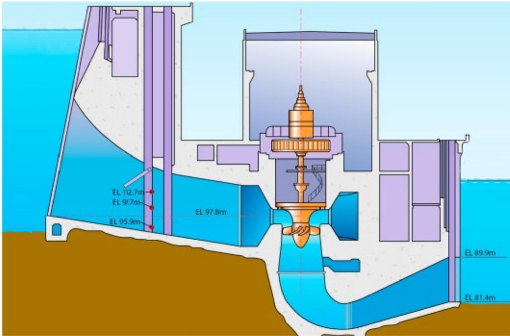
Figure 10: Schematic of a Kaplan turbine (used with permission) [56].
