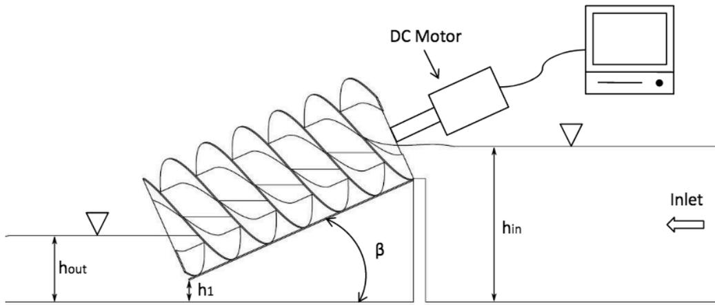
Figure 11: Schematic of an Archimedes turbine (used with permission) [57].
