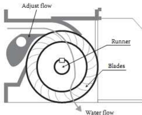
Figure 9: Schematic of a crossflow turbine. (used with permission) [55].
